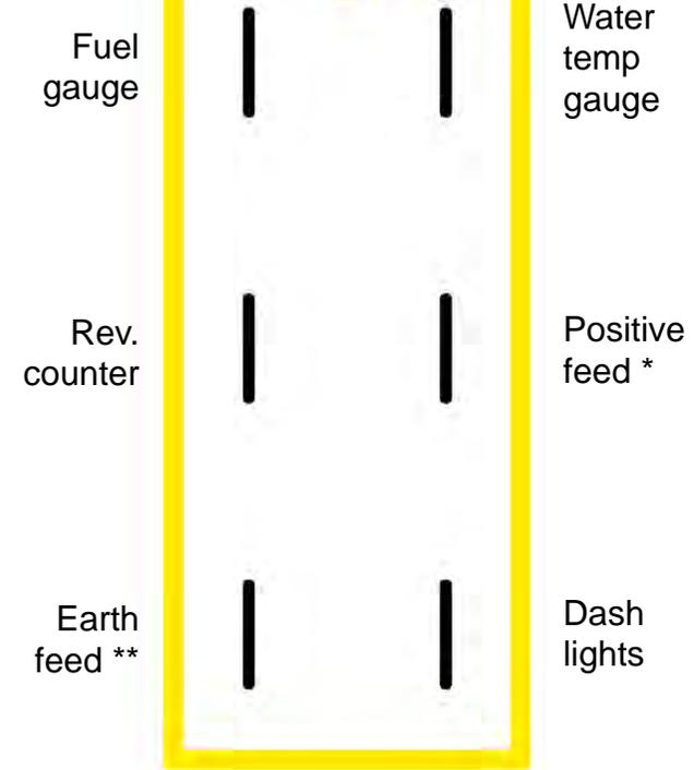
\* Positive feed for brake pads, temperature warning, temperature gauge, battery, brake hydraulics, oil, fuel.
